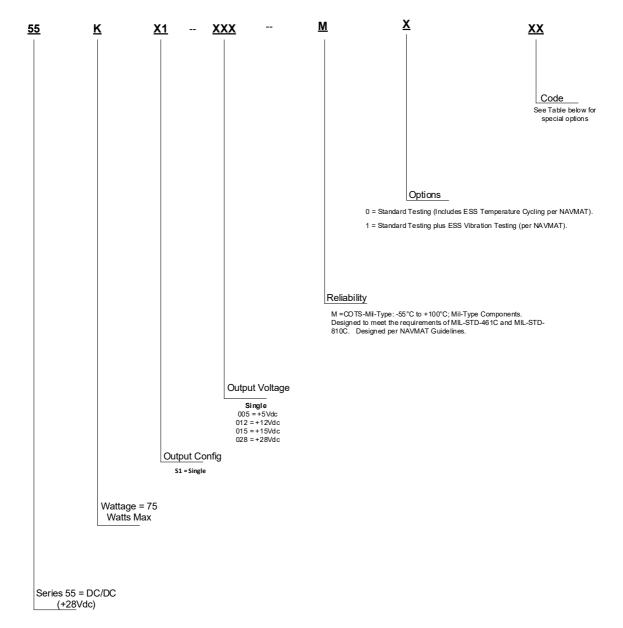
**Example:** 55KS1-028M0 = DC/DC (Low Voltage); 75 Watt; Single Output; +28V; COTS-MIL-Type; Standard Testing
